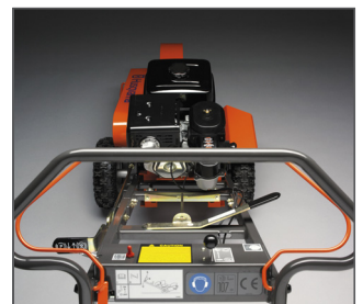
COMPACT DESIGN Compact design, needs only 70 cm/28" of lateral clearance.
