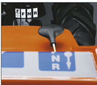
TWO GEARS One gear forward and one reverse, for easy operation.
